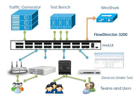
Additionally the FlowDirector provides total visibility into the network without impacting DUTs or test setup. The on-demand tapping capability has been proven to be useful for engineers and administrators to obtain information and diagnose the root cause.
